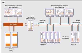
9 S+ Engineering Field Device Management Tools | 10 INFI-Net to Ethernet bridge (IEB800)
